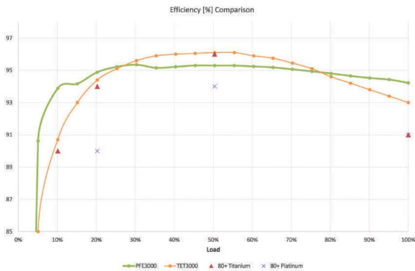
Efficiency curves for the Bel Power Platinum (PFE3000) and Titanium (TET3000) power supplies.
