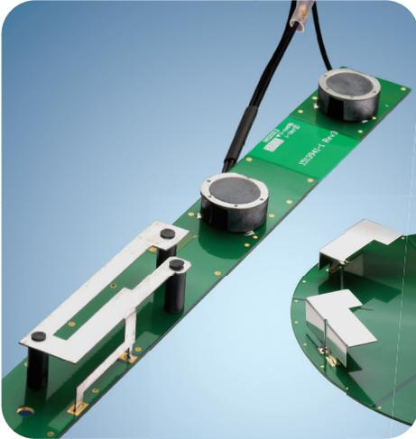
TE has developed a standard line of low profile, high performance stamped metal antenna solutions, and we can provide custom designs as well. Stamped metal antennas offer customers a low cost and highly repeatable manufacturing solution with a number of standard “off the shelf” or customized antenna designs. Stampings are a proven solution with several advantages such as:
