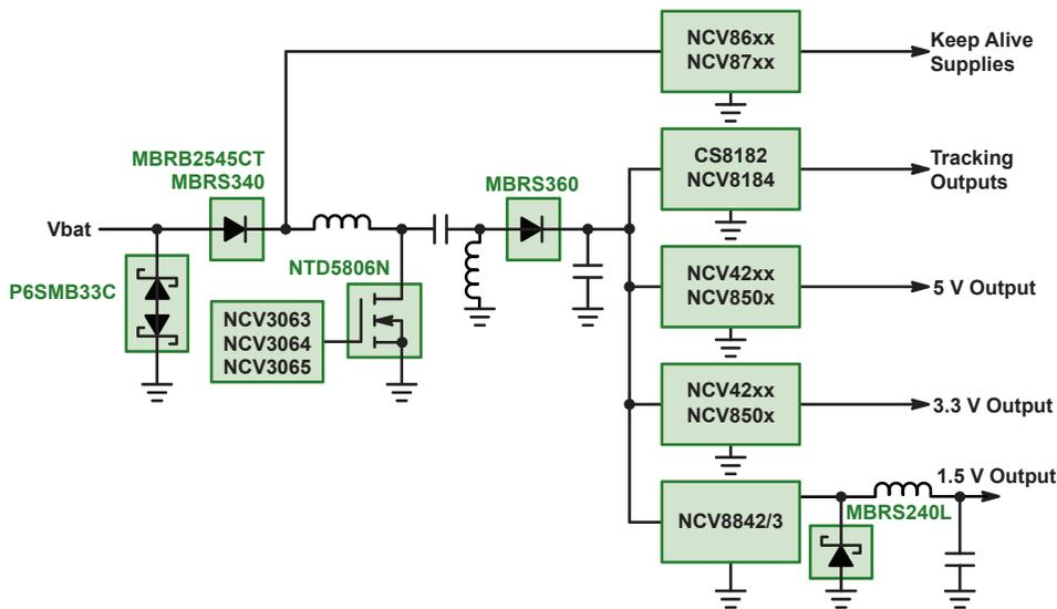
ON Semiconductor offers a wide selection of highly efficient power supply solutions that can handle harsh powertrain battery transients. The portfolio includes multi-topology controllers, such as NCV8871 and NCV3063, to provide regulated voltage greater than 5 V with a battery operating voltage between 4 V to 18 V; as well as buck regulators and controllers, like NCV8851 and NCV8842, to supply the high current, low voltage microcontroller cores.
