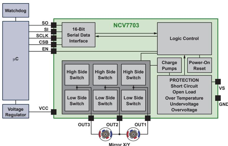
For mirror positioning, two motors adjust the glass along x and y axes. The NCV7703 features three integrated half-bridge drivers. The output stages are controlled by a 16-bit SPI interface. Complete diagnostic information is provided to the microcontroller through the SPI.
