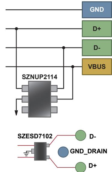
One High Speed Pair, V<sub>CC</sub>, Common Mode Filter + ESD Protection
