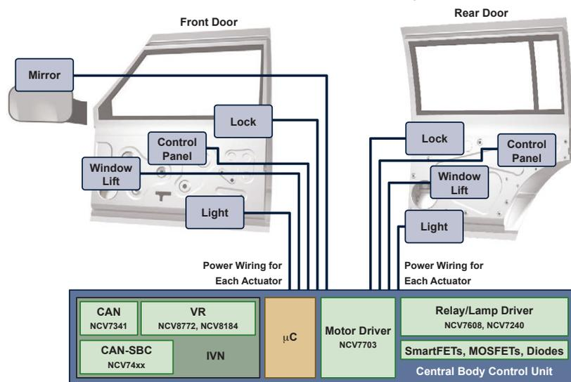
The most common topology is centralized electronics, where the electronics system is implemented in the Body Control Unit (BCU). ON Semiconductor offers:
