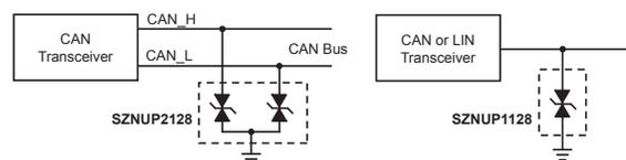
CAN and LIN protection devices improve the noise immunity and reliability of vehicular networks by suppressing overvoltage transients from conducted and radiated EMI and ESD.
