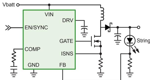
**NCV8871xx Backlighting PWM Deep Dimming Application - Minimal External Components**
