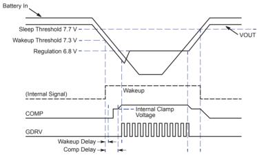
**Typical Output Waveforms Through Battery Cranking Profile**
