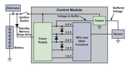
**Buffering Voltage to Send it Outside of a Module to a Sensor**
