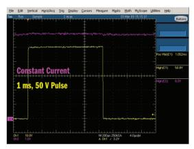
**Constant Current Supply During Vehicle Battery Load Dump**
