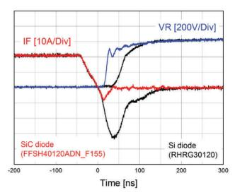
**Reverse Recovery & Leakage vs Temperature**
