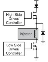
**Engine Control and Energy Recirculation Diodes**
