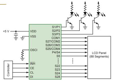
LC75843 Application Diagram, 1/4 Duty, 3-Channel PWM
