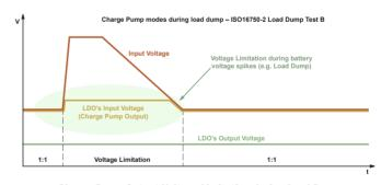
**Charge Pump Output Voltage Limitation during Load Dump**
