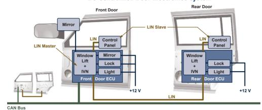
As the electronics content becomes more complex, the large amount of wires drives designs toward a de-centralized topology. The de-centralized door modules communicate over a CAN or LIN bus system.
