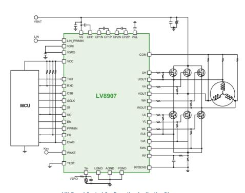
**LIN-Based Control Configuration Application Diagram**
