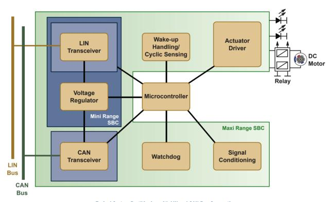
**Typical System Partitioning with LIN and CAN Bus Connections**
