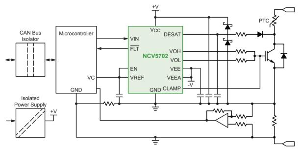
**PTC Heater Application Schematic**
