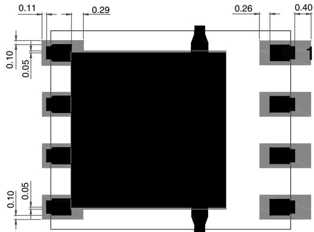
Overlap Flipped "PowerPAK SO-8 PCB Foot Print" onto "PowerPAK SO-8 Backside View"
