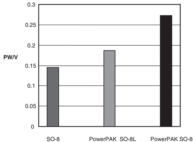
Fig. 4 - Thermal Fatigue Displacement Comparisons
