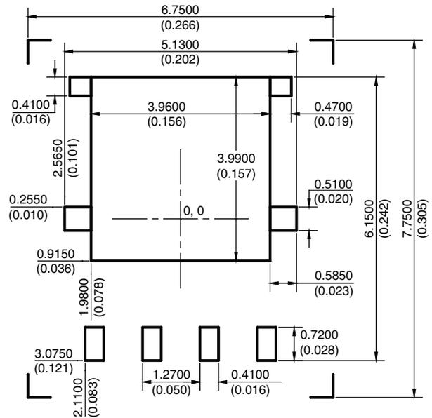
**Fig. 8 - Recommended PAD for Single Channel PowerPAK SO-8L**
