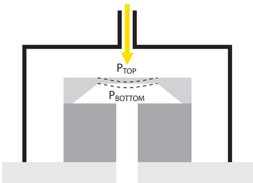
**Figure 1:** The top side pressure,  $P_{TOP}$ , must be higher than the gauge reference,  $P_{BOTTOM}$ , and results in positive change of differential output voltage of the pressure sensor. The gauge reference is identical to the local atmospheric pressure level.
