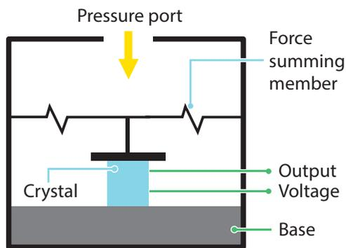
Figure 9: Piezoelectric sensor
