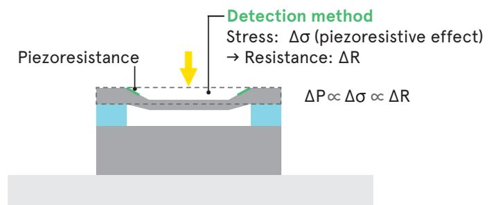
Figure 5: Schematic illustration of a piezoresistive element cross section
