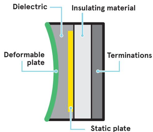
**Figure 8:** Capacitive sensor
