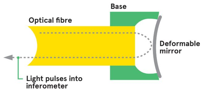
Figure 10: Optical sensor
