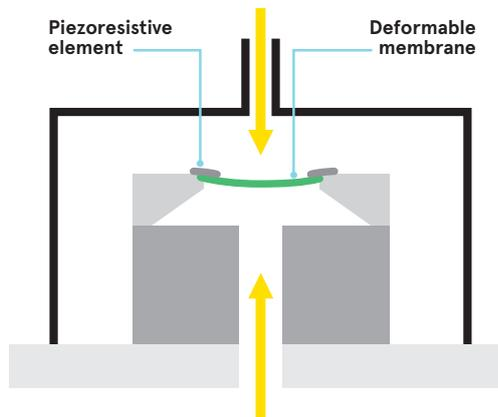
**Figure 7:** Piezoresistive sensor
