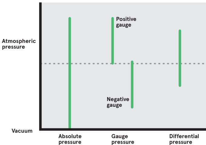
Figure 4: Differences in types of pressure measurement
