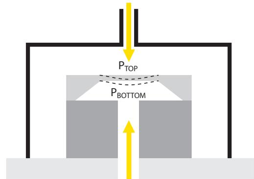
**Figure 3:** Differential pressure sensor. A top side pressure,  $P_{TOP}$ , higher than the bottom side pressure,  $P_{BOTTOM}$ , results in positive change of differential output voltage of the pressure sensor. Bottom side pressure being higher than top side pressure results in negative change of differential output voltage of the pressure sensor.
