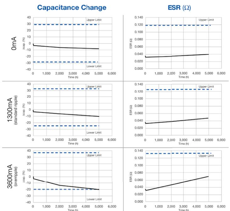
Hybrid capacitors exhibit high reliability when subjected to high ripple currents. In recent testing, the capacitors had the electrical characteristics at no load and rated ripple current (1,300mA) conditions. At three times the rated ripple current (3,600mA), the capacitor's electrical characteristics did change, but no shortage took place.
