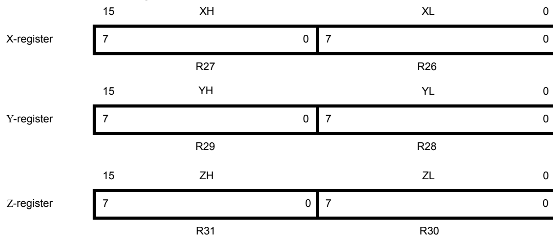
Figure 8-3. The X-, Y-, and Z-registers
