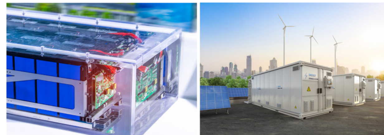
Figure 2: The range of energy storage systems extends from small battery systems (3 to 20 kWh, left) for households to large ones (100 kWh to 5 MWh, right) for grid operators (Source: Adobe Stock, right: phonlamaiphoto, left: xiaoliangge)
