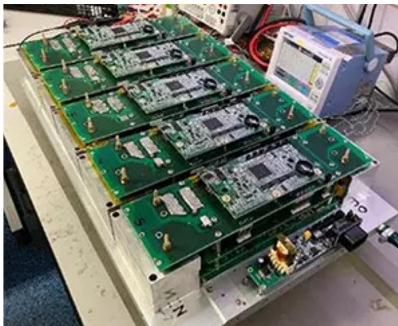
Figure 4: RECOM's Modular 5x15kW (75kW) Fuel Cell DC/DC Converter
