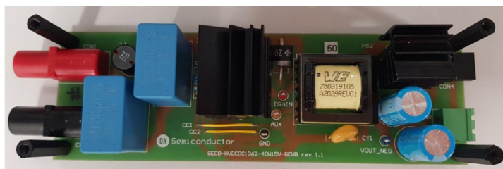
SiC Auxiliary Power Supply with NCV1362 controller
