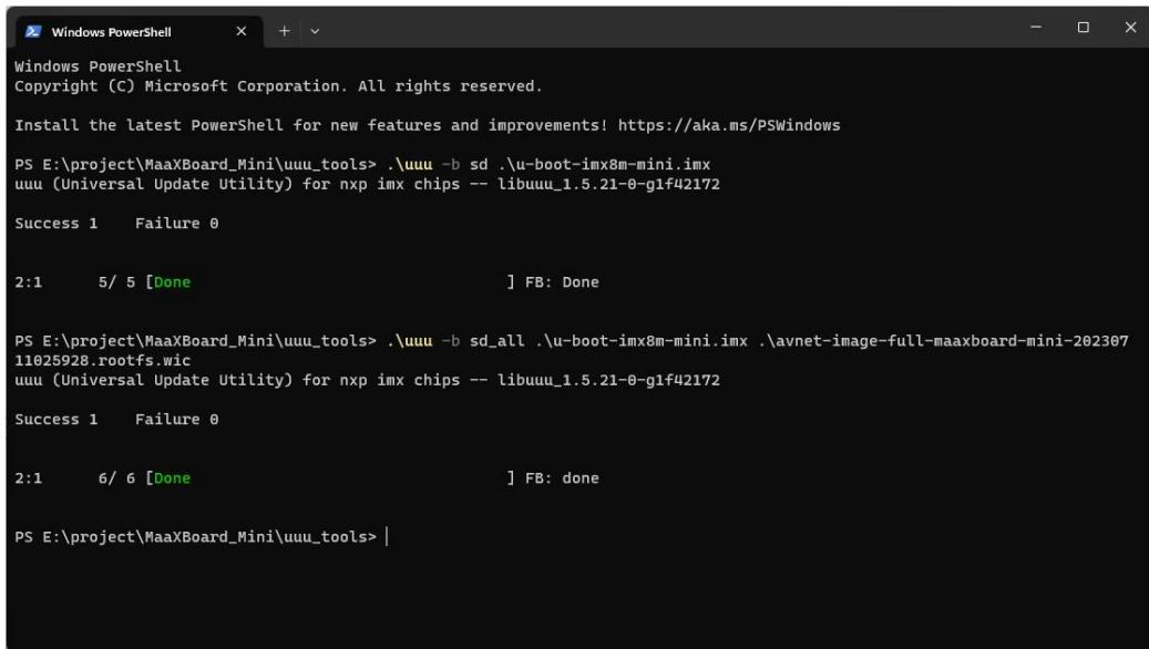
A screenshot of a Windows PowerShell window titled "Windows PowerShell". The window shows the command ".\uuu -b sd u-boot-imx8m-mini.imx" being run, followed by ".\\uuu -b sd\_all u-boot-imx8m-mini.imx" and "avnet-image-full-maaxboard-mini-20230711025928.rootfs.wic". The output indicates success for both operations, with counts of 1 success and 0 failures, and a total of 6 operations completed.
