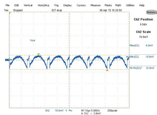
Figure 46: Output voltage ripple at 25A load Ch_2: V_{out}
