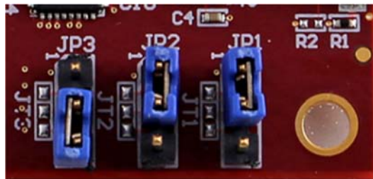
Figure 12 – MicroZed QSPI Boot Mode
