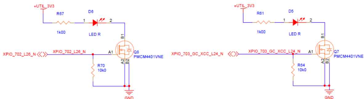
Figure 50 – XPIO LEDs Schematic
