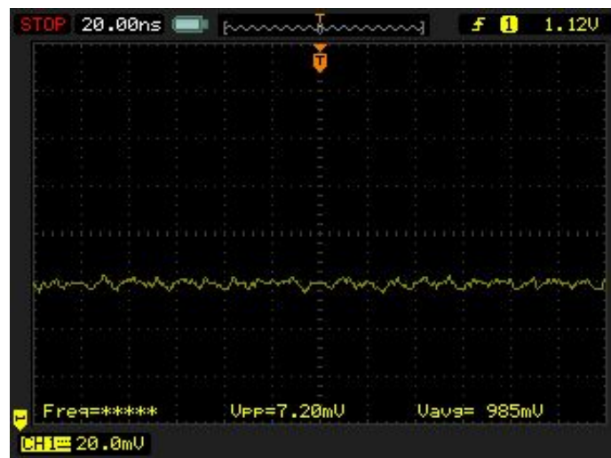
Figure 19 – 1V (Vccbram) measured across C348 – 7.2mV
