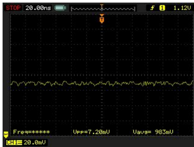
Figure 17 – 1V (Vccint) measured across C357 – 7.2mV
