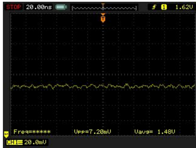
Figure 15 – 1.5V measured across C480 – 7.2mV
