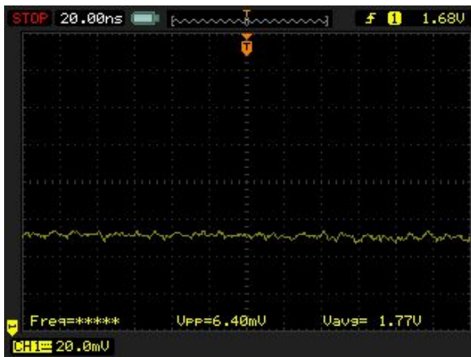
Figure 20 – 1.8V (Vccmio) measured across C344 – 6.4mV
