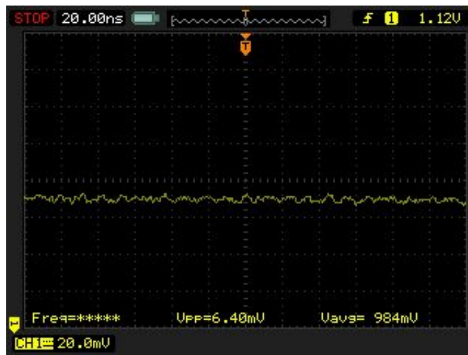
Figure 16 – 1V (Vccpint) measured across C366 – 6.4mV
