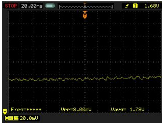
Figure 18 – 1.8V (Vccpaux) measured across C222 – 8.0mV
