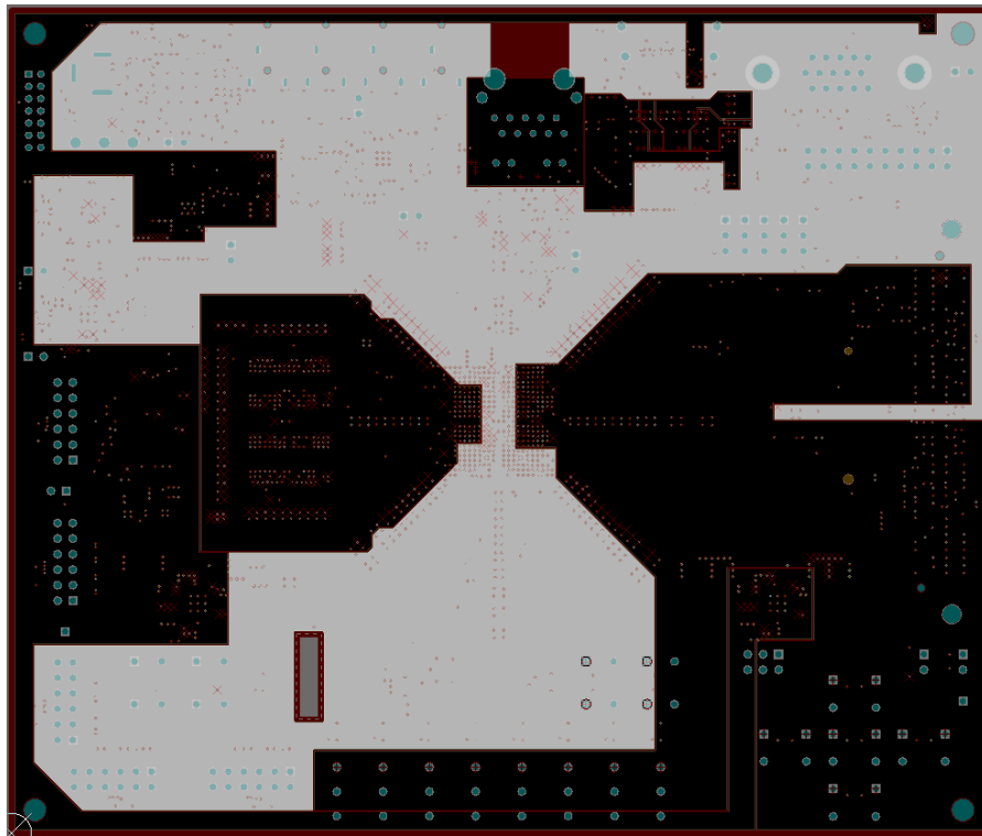
Figure 1 – Power Plane one 1.8V Vccaux Flood
