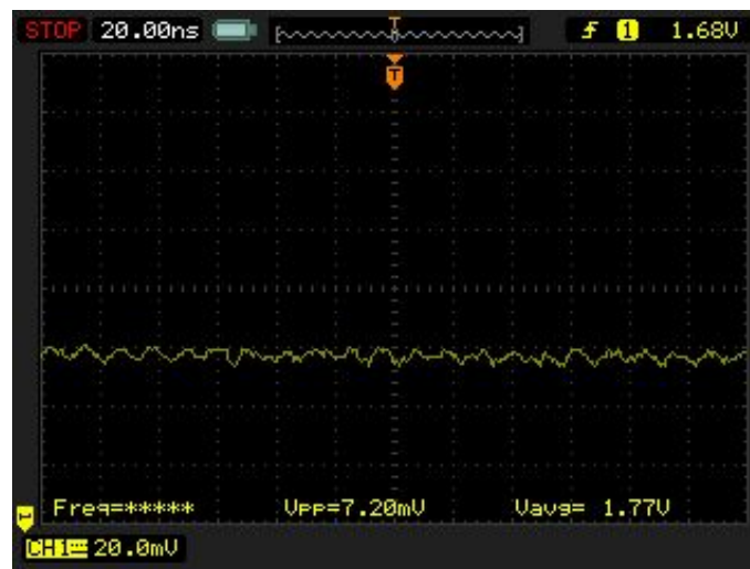
Figure 14 – 1.8V (Vccpau) measured across C339 – 7.2mV
