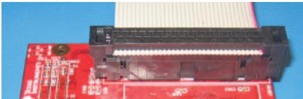
Figure 13 – Connecting the image sensor's flat cable (2 of 2)
