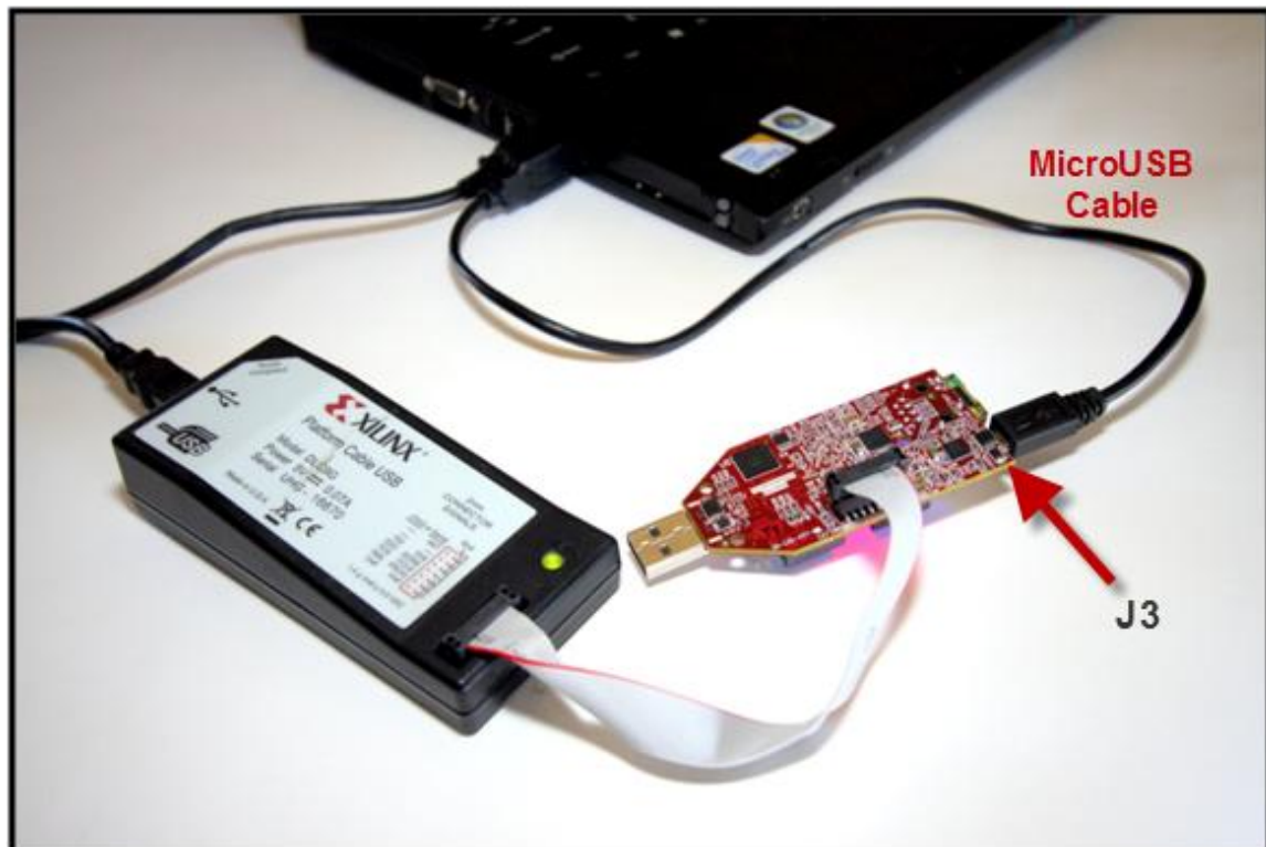
Figure 16 - Configuration Setup with Xilinx Platform Cable USB
