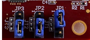
Figure 48 – SD Card Boot Jumper Settings
