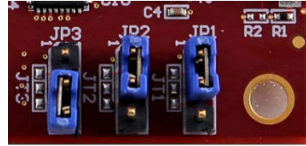
Figure 4 – MicroZed Jumper Settings
