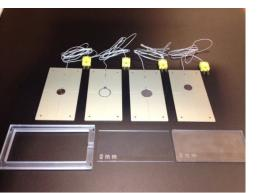
The Qi Foreign Objects are WPC defined metal objects that can be placed between Qi wireless transmitters and receivers and used to evaluate the FOD operation and performance.
