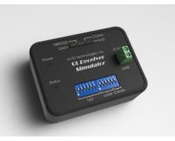
The Qi Receiver Simulator is a low power receiver that can be used to test the operation and performance of Qi wireless power transmitters. DIP switches on top of the Qi Receiver Simulator can be used to select different operational test modes as well as select different communication modulators and internal loads.
