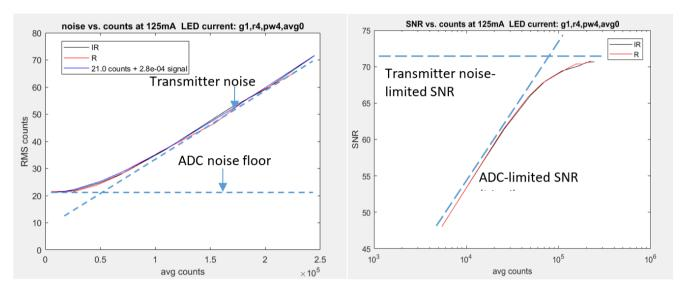
Figure 5. SNR vs. Signal Level
