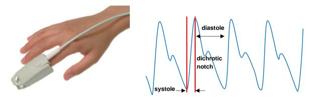
Figure 2. Finger Clip-based Transmission PPG
