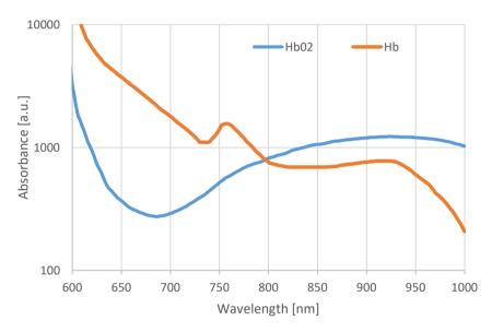
Figure 4. Absorbance Spectra for Oxyhemoglobin (HbO2) and Deoxyhemoglobin (Hb)
