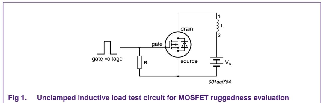
Fig 1. Unclamped inductive load test circuit for MOSFET ruggedness evaluation
