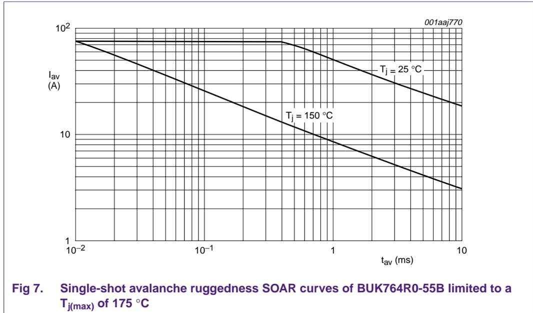
**Figure 7** shows the SOAR curves of a device single-shot avalanche capability. The 25 °C junction temperature curve shows the maximum allowable  $I_{AS}$  for a given  $t_{AV}$  at an initial  $T_j$  of 25 °C. This maximum  $I_{AV}$  will give rise to a maximum junction temperature,  $T_{jrise(max)}$  of 150 °C resulting in a  $T_{j(max)}$  of 175 °C.
