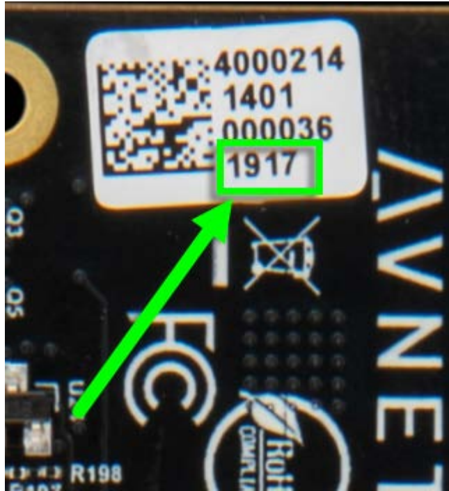
Figure 2 – Datecode of 1917 is 17 th week of 2019, which is week of April 21st
