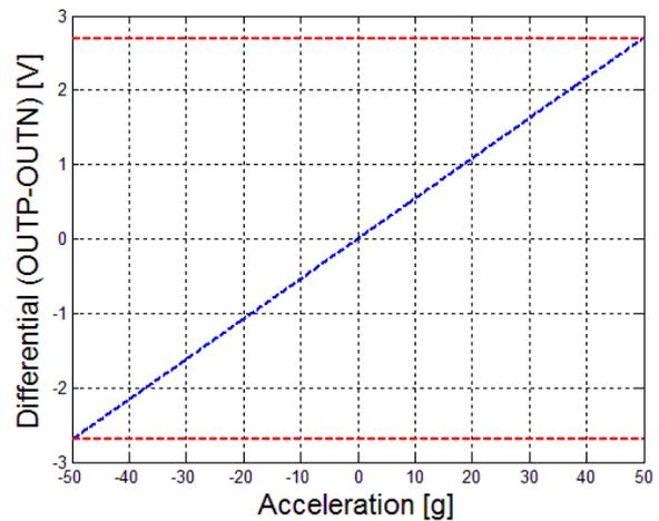
Figure 25: Differential acceleration output (OUTP-OUTN) at full scale
