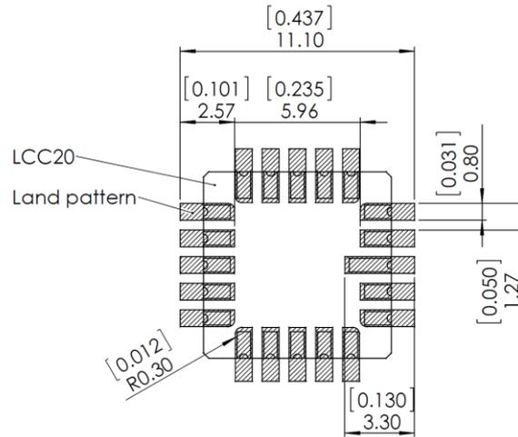
Figure 45 : LCC20 land pattern recommendation (unit are mm/[inch])
