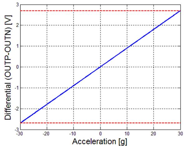
Figure 20: Differential acceleration output (OUTP-OUTN) at full scale
