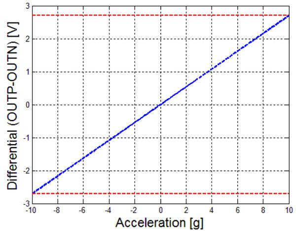
Figure 15: Differential acceleration output (OUTP-OUTN) at full scale
