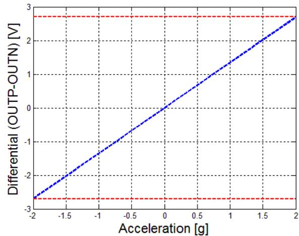
Figure 4: Differential acceleration output (OUTP-OUTN) at full scale
