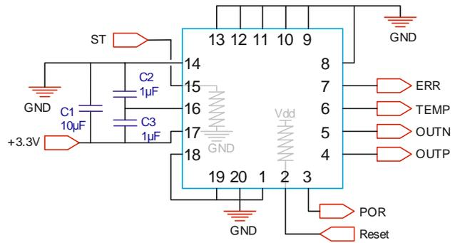
Figure 38: Proximity circuit & pull-up/down
