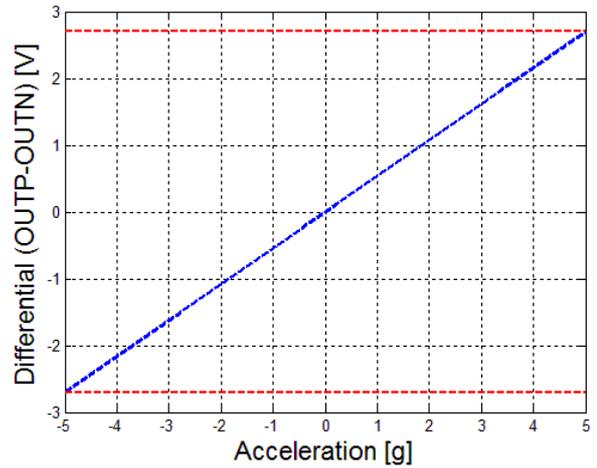
Figure 10: Differential acceleration output (OUTP-OUTN) at full scale
