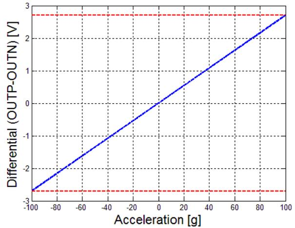
Figure 30: Differential acceleration output (OUTP-OUTN) at full scale
