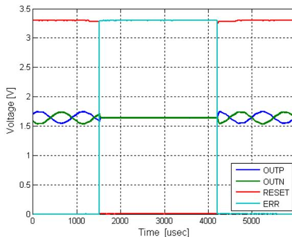
Figure 40: Typical sensor reset sequence with external reset
