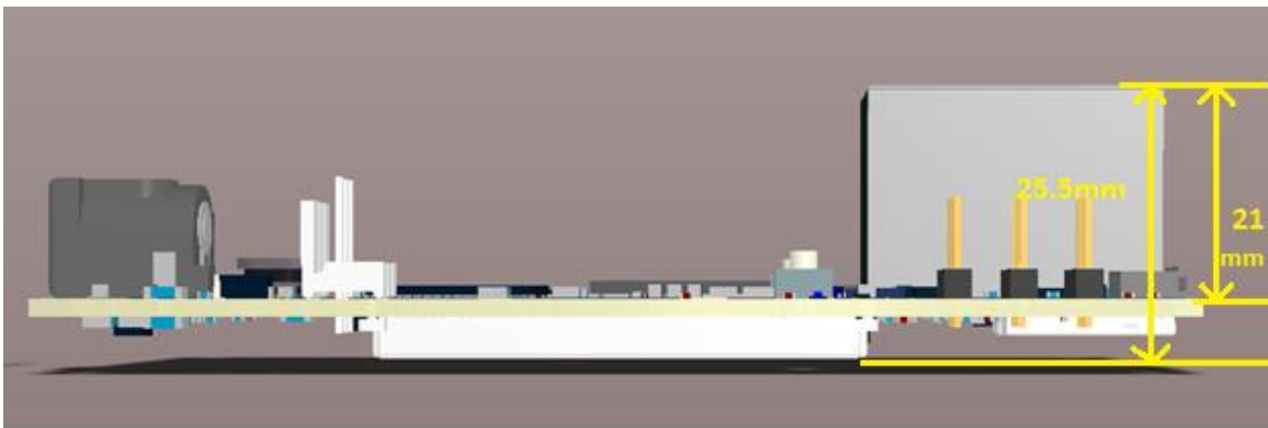
Figure 6 – MicroZed Side Vertical Dimensions (Side)
