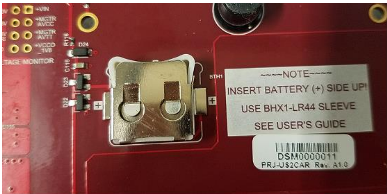
Figure 53 – Final battery placement. Push battery in as far as possible.
