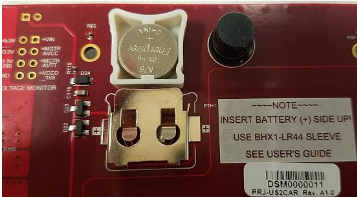
Figure 52 – Battery & sleeve orientation prior to insertion
