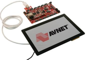
11. Turn I/O Carrier Card power switch (SW5) ON. The green Power Good LED (D5) on MicroZed and the green Power Good LED (LED10) should illuminate.
