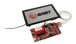
11. Turn FMC Carrier Card power switch (SW3) ON. The green Power Good LED (D5) on MicroZed and the green Power Good LED (LED6) should illuminate.
