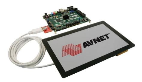
Turn ZedBoard power switch (SW8) ON. The green POWER LED (LD13) on ZedBoard should illuminate. 11. After about 2 seconds, the blue DONE LED (LD12) on ZedBoard should illuminate and the "Configuring System Please Wait" screen should appear.
