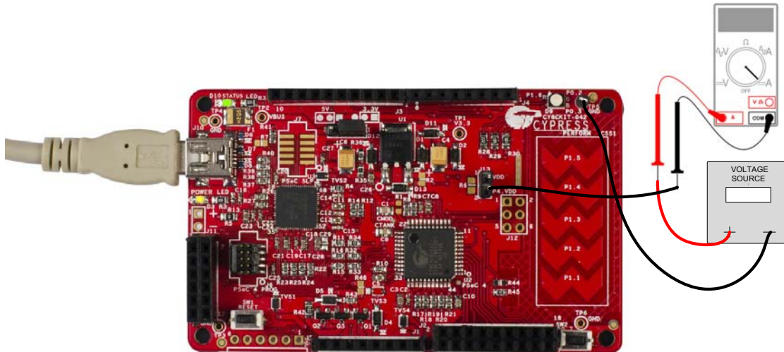
Figure 4-6. PSoC 4 Current Measurement when Powered Separately
