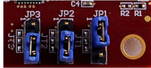
Figure 55 – SD Card Boot Jumper Settings
